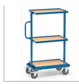
Tubular steel and steel section construction, powder coated. With 3 platforms made of derived timber material boards, rim 10 mm high. Capacity upper and middle shelf 50 kg. 2 swivel and 2 fixed-wheel castors, TPE tyres, 125 x 32 mm, hubs with groove ball bearing. Swivel castors with wheel lock, according to European Standard EN1757-3 (safety of platform trolleys).
