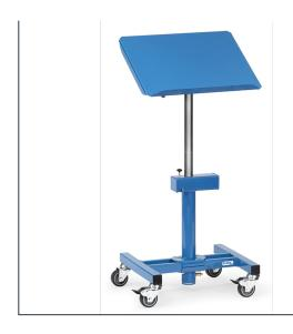
For plastic boxes, steel plate boxes, wire baskets etc., adjustable in height and mobile. Sectional steel-/ tubular construction with steel plate platform. Powder-coated blue RAL 5007. 4 swivel castors with TPE tyres, hubs with bush bearing, 2 swivel castors with wheel locks. Steel plate platform with single-sided lay-on edge, inclinable by 15° and 30°, continuously adjustable in height, rotatable and lockable, with pneumatic lowering damping.
