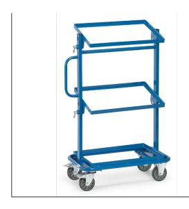
Tubular steel and steel section construction, powder coated. Upper and middle surface tiltable to both sides by 15° and 30°, locked by spring catch. With open frames without board. Capacity upper and middle shelf 50 kg. 2 swivel and 2 fixed-wheel castors, TPE tyres, 125 x 32 mm, hubs with groove ball bearing. Swivel castors with wheel lock, according to European Standard EN1757-3 (safety of platform trolleys).
