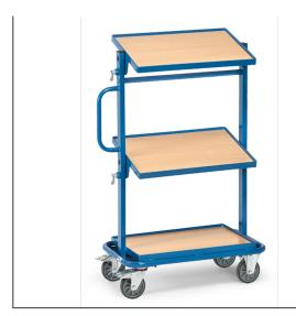
Tubular steel and steel section construction, powder coated. Upper and middle surface tiltable to both sides by 15° and 30°, locked by spring catch. With 3 platforms made of derived timber material boards, rim 10 mm high. Capacity upper and middle shelf 50 kg. 2 swivel and 2 fixed-wheel castors, TPE tyres, 125 x 32 mm, hubs with groove ball bearing. Swivel castors with wheel lock, according to European Standard EN1757-3 (safety of platform trolleys).
