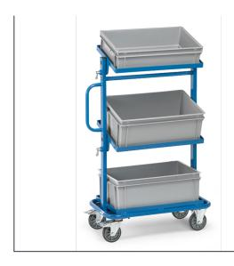
Tubular steel and steel section construction, powder coated. Upper and middle surface tiltable to both sides by 15° and 30°, locked by spring catch. With 6 plastic boxes, 2 pc. 600 x 400 x 145 mm 4 pcs. 600 x 400 x 220 mm. Capacity upper and middle shelf 50 kg. 2 swivel and 2 fixed-wheel castors, TPE tyres, 125 x 32 mm, hubs with groove ball bearing. Swivel castors with wheel lock, according to European Standard EN1757-3 (safety of platform trolleys).
