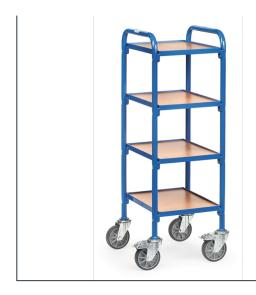
Modular system: Tubular steel and steel section construction, powder coated. Capacity per shelf 50 kg. 4 shelves of derived timber board, rim 12 mm high. 4 castors with TPE tyres, hubs with groove ball bearing, 2 wheels with locks, according to European Standard EN1757-3 (safety of platform trolleys).
