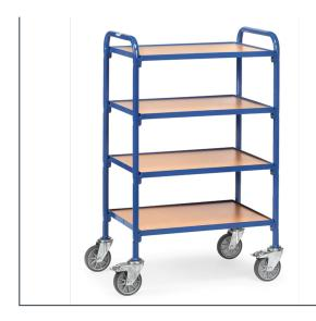
Modular system: Tubular steel and steel section construction, powder coated. Capacity per shelf 50 kg. 4 shelves of derived timber board, rim 12 mm high. 4 castors with TPE tyres, hubs with groove ball bearing, 2 wheels with locks, according to European Standard EN1757-3 (safety of platform trolleys).
