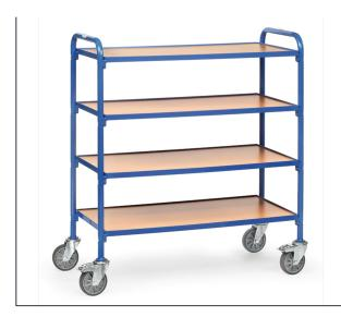
Modular system: Tubular steel and steel section construction, powder coated. Capacity per shelf 50 kg. 4 shelves of derived timber board, rim 12 mm high. 4 castors with TPE tyres, hubs with groove ball bearing, 2 wheels with locks, according to European Standard EN1757-3 (safety of platform trolleys).
