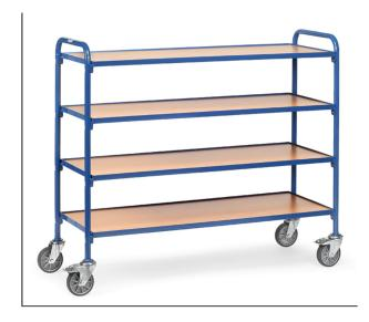
Modular system: Tubular steel and steel section construction, powder coated. Capacity per shelf 50 kg. 4 shelves of derived timber board, rim 12 mm high. 4 castors with TPE tyres, hubs with groove ball bearing, 2 wheels with locks, according to European Standard EN1757-3 (safety of platform trolleys).
