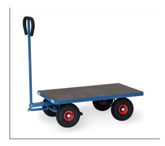
Made of tubular steel, welded and powder coated blue RAL 5007. Platform made of waterresistant plywood. Bogie steering with shaft and handle. Wheels with pneumatic tyres, hubs with roller bearings. Shaft with safety handle and with an automatic damped retraction in resting position. With automatic breaking system effective on the front wheels according to the European Standard EN 1757-3.
