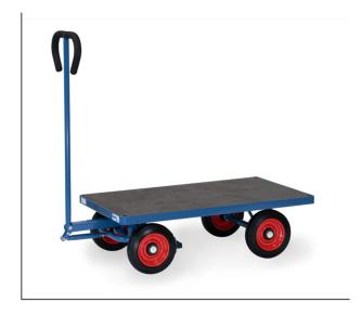
Made of tubular steel, welded and powder coated blue RAL 5007. Platform made of waterresistant plywood. Bogie steering with shaft and handle. Wheels with solid rubber tyres, hubs with roller bearings. Shaft with safety handle and with an automatic damped retraction in resting position. With automatic breaking system effective on the front wheels according to the European Standard EN 1757-3.
