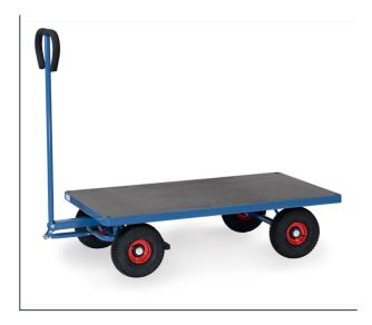
Made of tubular steel, welded and powder coated blue RAL 5007. Platform made of waterresistant plywood. Bogie steering with shaft and handle. Wheels with pneumatic tyres, hubs with roller bearings. Shaft with safety handle and with an automatic damped retraction in resting position. With automatic breaking system effective on the front wheels according to the European Standard EN 1757-3.
