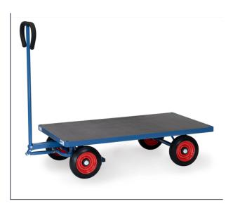
Made of tubular steel, welded and powder coated blue RAL 5007. Platform made of waterresistant plywood. Bogie steering with shaft and handle. Wheels with solid rubber tyres, hubs with roller bearings. Shaft with safety handle and with an automatic damped retraction in resting position. With automatic breaking system effective on the front wheels according to the European Standard EN 1757-3.
