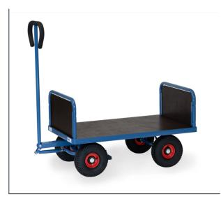
Made of tubular steel, welded and powder coated blue RAL 5007. Platform made of waterresistant plywood. With two ends 300 mm high. Tubular steel frame with waterresistant plywood. Bogie steering with shaft and handle. Wheels with pneumatic tyres, hubs with roller bearings. Shaft with safety handle and with an automatic damped retraction in resting position. With automatic breaking system effective on the front wheels according to the European Standard EN 1757-3.
