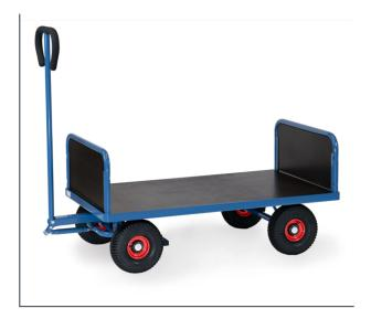
Made of tubular steel, welded and powder coated blue RAL 5007. Platform made of waterresistant plywood. With two ends 300 mm high. Tubular steel frame with waterresistant plywood. Bogie steering with shaft and handle. Wheels with pneumatic tyres, hubs with roller bearings. Shaft with safety handle and with an automatic damped retraction in resting position. With automatic breaking system effective on the front wheels according to the European Standard EN 1757-3.
