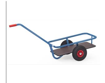
Light hand cart with plastic tray. Tubular steel and steel section construction, powder coated blue RAL 5007. Shaft with 1 handle. Shaft can be screwed on. Wheels with pneumatic tyres, hubs with roller bearings. Platform made of water-resistant plywood boards. Flat packed for easy self assembly.
