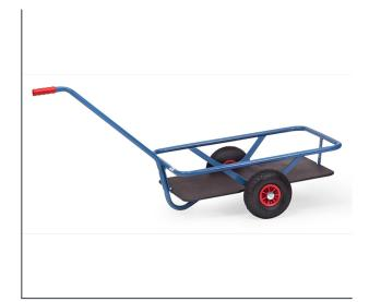
Light hand cart with plastic tray. Tubular steel and steel section construction, powder coated blue RAL 5007. Shaft with 1 handle. Shaft can be screwed on. Wheels with pneumatic tyres, hubs with roller bearings. Platform made of water-resistant plywood boards. Flat packed for easy self assembly.
