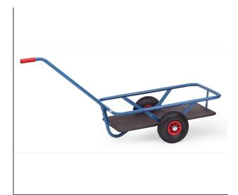
Light hand cart with plastic tray. Tubular steel and steel section construction, powder coated blue RAL 5007. Shaft with 1 handle. Shaft can be screwed on. Wheels with solid rubber tyres, hubs with roller bearings. Platform made of water-resistant plywood boards. Flat packed for easy self assembly.
