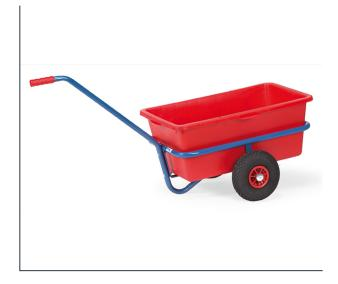
Light hand cart with plastic tray. Tubular steel and steel section construction, powder coated blue RAL 5007. Shaft with 1 handle. Wheels with pneumatic tyres, hubs with roller bearings. Plastic tray, red, contents 90 litres. Flat packed for easy self assembly. 4101: L x W x H = 715 x 420 x 320 mm.
