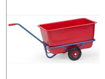
Light hand cart with plastic tray. Tubular steel and steel section construction, powder coated blue RAL 5007. Shaft with 1 handle. Wheels with pneumatic tyres, hubs with roller bearings. Plastic tray, red, contents 90 litres. Flat packed for easy self assembly. 4102: L x W x H = 990 x 665 x 476 mm.
