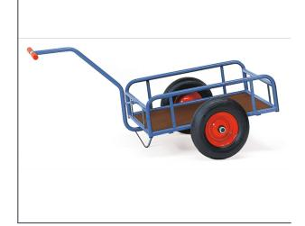
Made of tubular steel, welded and powder coated. Rail 250 mm high, shaft bolted on. Platform made of water-resistant plywood boards. Wheels with solid rubber tyres, hubs with roller bearings. Accessories for hand carts: Coupling for bicycles.
