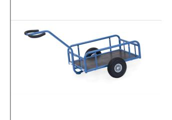
Made of tubular steel, welded and powder coated. Rail 250 mm high, shaft bolted on. Platform made of water-resistant plywood boards. Wheels with pneumatic tyres, hubs with roller bearings. Accessories for hand carts: Coupling for bicycles.
