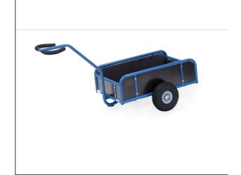
Made of tubular steel, welded and powder coated. Rail 250 mm high, shaft bolted on. Platform made of water-resistant plywood boards. Wheels with pneumatic tyres, hubs with roller bearings. With waterproof box superstructure made of plywood, 250 mm high.
