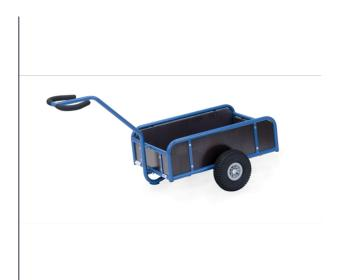
Made of tubular steel, welded and powder coated. Rail 250 mm high, shaft bolted on. Platform made of water-resistant plywood boards. Wheels with pneumatic tyres, hubs with roller bearings. With waterproof box superstructure made of plywood, 250 mm high.
