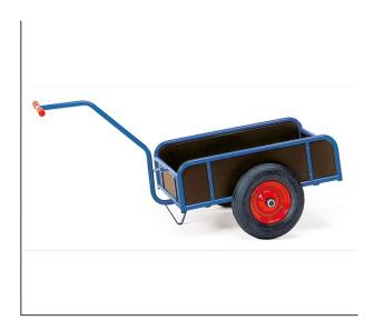
Made of tubular steel, welded and powder coated. Rail 250 mm high, shaft bolted on. Platform made of water-resistant plywood boards. Wheels with solid rubber tyres, hubs with roller bearings. With waterproof box superstructure made of plywood, 250 mm high.
