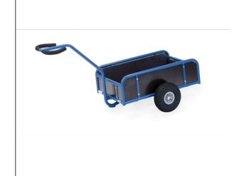
Made of tubular steel, welded and powder coated. Rail 250 mm high, shaft bolted on. Platform made of water-resistant plywood boards. Wheels with pneumatic tyres, hubs with roller bearings. With waterproof box superstructure made of plywood, 250 mm high.
