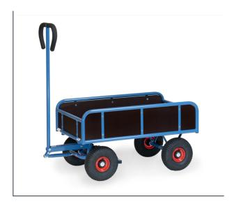
Made of tubular steel, welded and powder coated. Rail 250 mm high, platform, sides and ends made of water-resistant plywood. Bogie steering with shaft and handle. Wheels with pneumatic tyres, hubs with roller bearings. Shaft with safety handle and with an automatic damped retraction in resting position. With automatic braking system effective on the front wheels according to the European Standard EN 1757-3.
