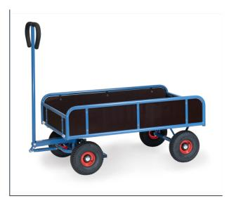
Made of tubular steel, welded and powder coated. Rail 250 mm high, platform, sides and ends made of water-resistant plywood. Bogie steering with shaft and handle. Wheels with pneumatic tyres, hubs with roller bearings. Shaft with safety handle and with an automatic damped retraction in resting position. With automatic braking system effective on the front wheels according to the European Standard EN 1757-3.
