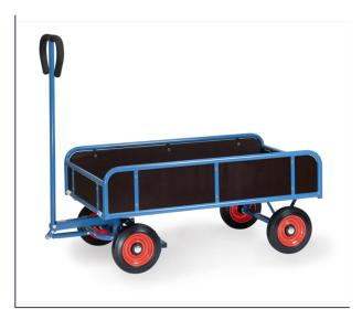
Made of tubular steel, welded and powder coated. Rail 250 mm high, platform, sides and ends made of water-resistant plywood. Bogie steering with shaft and handle. Wheels with solid rubber tyres, hubs with roller bearings. Shaft with safety handle and with an automatic damped retraction in resting position. With automatic braking system effective on the front wheels according to the European Standard EN 1757-3.
