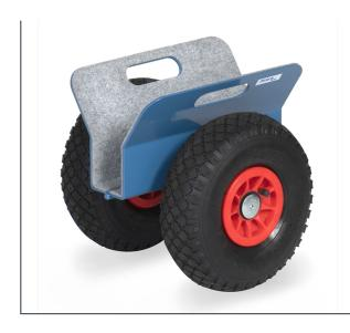
Steel-welded construction, powder coated blue RAL 5007. Jaw surface with felt coating. Wheels with pneumatic tyres, hubs with roller bearings. Secure clamping by the weight of the load on the clamping construction. Maximal clamping width: 0-60 mm.
