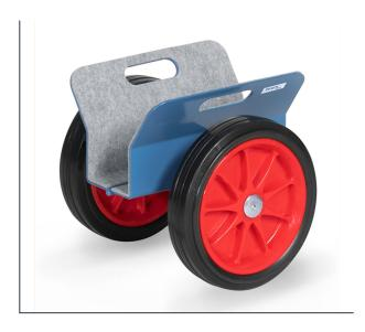
Steel-welded construction, powder coated blue RAL 5007. Jaw surface with felt coating. Wheels with solid rubber tyres, hubs with roller bearings. Secure clamping by the weight of the load on the clamping construction. Clamping width 30-95 mm (suitable for windows).
