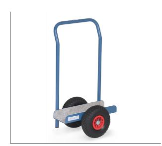
Steel sheet construction, powder coated blue RAL 5007, interior surface with felt coating. Wheels with solid rubber tyres, hubs with roller bearings. With support and push bar. Clear width: 150 mm.
