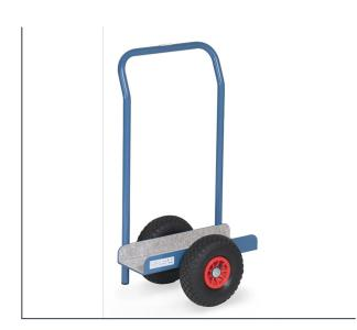
Steel sheet construction, powder coated blue RAL 5007, interior surface with felt coating. Wheels with pneumatic tyres, hubs with roller bearings. With support and push bar. Total height: 900 mm. Clear width: 150 mm.
