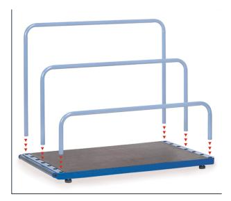
Welded sectional and tubular steel, powder coated, with wooden platform. 7 positions for insertable tubular supports. 4 rubber feet, floor anchoring possible. One face end fitted with 6-pieces of pick-up rolls. For up to 1200 kg capacity Delivery without tubular supports. Clearance between tubular supports 90 mm.
