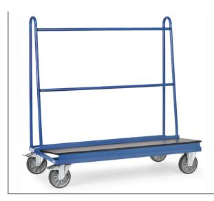
Welded profile steel and steel tube. Anti-skid loading platform of waterproof plywood. 2 swivel and 2 fixed-wheel castors, TPE tyres, hubs with groove ball bearing. Swivel castors with wheel locks, according to the European Standard EN 1757-3 (safety of platform trolleys).
