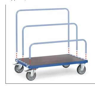
Welded sectional and tubular steel, powder coated, with wooden platform. 7 positions for insertable tubular supports. Clearance between supports 90 mm. 2 swivel and 2 fixed-wheel castors. Swivel castors wheels with wheel lock, according to the European Standard EN 1757-3 (safety of platform trolleys).
