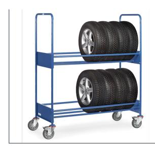
Tubular steel construction, screwed together, powder coated blue RAL 5007. Tyre carrier variable adjustable in intervals of 150 mm with clamps on the face ends. 4 swivel castors with TPE tyres, hubs with groove ball bearing. 2 swivel castors with wheel locks.
