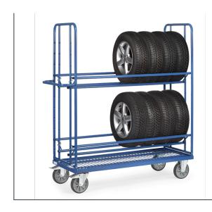
Tubular steel and steel section construction, powder coated. Shelves with welded wire lattice 140 x 40 mm. Carriers variably insertable within a distance of 120 mm. Due to the joint-like attachment, the carriers adapt automatically to the tyre size. 2 swivel and 2 fixed-wheel castors, TPE tyres, hubs with groove ball roller bearings. Swivel castors with wheel locks.
