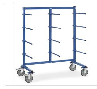
Modular system: Frame made of sturdy square tube. Cross beams, posts and bars connected with solid screwed joints. Carrier spars made of tubular steel Ø 27 mm with screwed joints. With 12 one-side carrier spars. Carrying capacity per level 80 kg. Powder coated blue RAL 5007. 2 swivel and 2 fixed-wheel castors, TPE tyres, hubs with groove ball bearing. Swivel castors with wheel locks, according to EN 1757-3.
