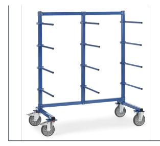
Modular system: Frame made of sturdy square tube. Cross beams, posts and bars connected with solid screwed joints. Carrier spars made of tubular steel Ø 27 mm with screwed joints. With 12 one-side carrier spars coated with PVC hose. Carrying capacity per level 80 kg. Powder coated blue RAL 5007. 2 swivel and 2 fixed-wheel castors, TPE tyres, hubs with groove ball bearing. Swivel castors with wheel locks, according to EN 1757-3.
