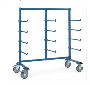
Modular system: Frame made of sturdy square tube. Cross beams, posts and bars connected with solid screwed joints. Carrier spars made of tubular steel Ø 27 mm with screwed joints. With 12 one-side carrier spars coated with PVC hose and with anti skidding device. Carrying capacity per level 80 kg. Powder coated blue RAL 5007. 2 swivel and 2 fixed-wheel castors, TPE tyres, hubs with groove ball bearing. Swivel castors with wheel locks, according to EN 1757-3.
