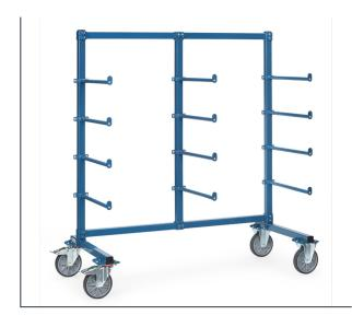
Modular system: Frame made of sturdy square tube. Cross beams, posts and bars connected with solid screwed joints. Carrier spars made of tubular steel Ø 27 mm with screwed joints. With 12 one-side carrier spars with anti skidding device. Carrying capacity per level 80 kg. Powder coated blue RAL 5007. 2 swivel and 2 fixed-wheel castors, TPE tyres, hubs with groove ball bearing. Swivel castors with wheel locks, according to EN 1757-3.
