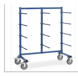
Modular system: Frame made of sturdy square tube. Cross beams, posts and bars connected with solid screwed joints. Carrier spars made of tubular steel Ø 27 mm with screwed joints. With 12 one-side carrier spars. Carrying capacity per level 80 kg. Powder coated blue RAL 5007. 2 swivel and 2 fixed-wheel castors, TPE tyres, hubs with groove ball bearing. Swivel castors with wheel locks, according to EN 1757-3.
