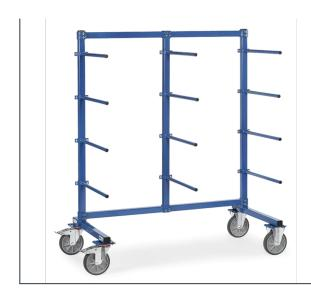
Modular system: Frame made of sturdy square tube. Cross beams, posts and bars connected with solid screwed joints. Carrier spars made of tubular steel Ø 27 mm with screwed joints. With 12 one-side carrier spars coated with PVC hose. Carrying capacity per level 80 kg. Powder coated blue RAL 5007. 2 swivel and 2 fixed-wheel castors, TPE tyres, hubs with groove ball bearing. Swivel castors with wheel locks, according to EN 1757-3.
