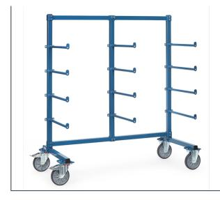
Modular system: Frame made of sturdy square tube. Cross beams, posts and bars connected with solid screwed joints. Carrier spars made of tubular steel Ø 27 mm with screwed joints. With 12 one-side carrier spars coated with PVC hose and with anti skidding device. Carrying capacity per level 80 kg. Powder coated blue RAL 5007. 2 swivel and 2 fixed-wheel castors, TPE tyres, hubs with groove ball bearing. Swivel castors with wheel locks, according to EN 1757-3.
