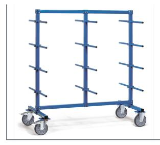
Modular system: Frame made of sturdy square tube. Cross beams, posts and bars connected with solid screwed joints. Carrier spars made of tubular steel Ø 27 mm with screwed joints. With 24 carrier spars on both sides (12 per side) coated with PVC hose. Carrying capacity per level 120 kg (60 kg per side). Powder coated blue RAL 5007. 2 swivel and 2 fixed-wheel castors, TPE tyres, hubs with groove ball bearing. Swivel castors with wheel locks, according to EN 1757-3.
