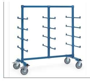
Modular system: Frame made of sturdy square tube. Cross beams, posts and bars connected with solid screwed joints. Carrier spars made of tubular steel Ø 27 mm with screwed joints. With 24 carrier spars on both sides (12 per side) coated with PVC hose and with anti skidding device. Carrying capacity per level 120 kg (60 kg per side). Powder coated blue RAL 5007. 2 swivel and 2 fixed-wheel castors, TPE tyres, hubs with groove ball bearing. Swivel castors with wheel locks, according to EN 1757-3.
