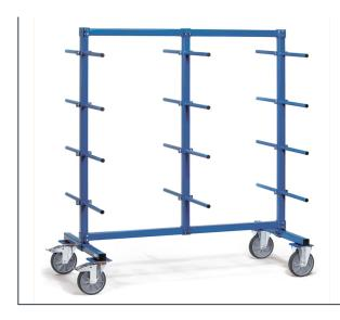
Modular system: Frame made of sturdy square tube. Cross beams, posts and bars connected with solid screwed joints. Carrier spars made of tubular steel Ø 27 mm with screwed joints. With 24 carrier spars on both sides (12 per side). Carrying capacity per level 120 kg (60 kg per side). Powder coated blue RAL 5007. 2 swivel and 2 fixed-wheel castors, TPE tyres, hubs with groove ball bearing. Swivel castors with wheel locks, according to EN 1757-3.
