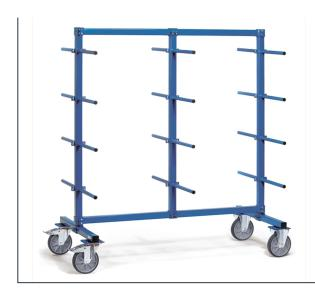
Modular system: Frame made of sturdy square tube. Cross beams, posts and bars connected with solid screwed joints. Carrier spars made of tubular steel Ø 27 mm with screwed joints. With 24 carrier spars on both sides (12 per side) coated with PVC hose. Carrying capacity per level 120 kg (60 kg per side). Powder coated blue RAL 5007. 2 swivel and 2 fixed-wheel castors, TPE tyres, hubs with groove ball bearing. Swivel castors with wheel locks, according to EN 1757-3.
