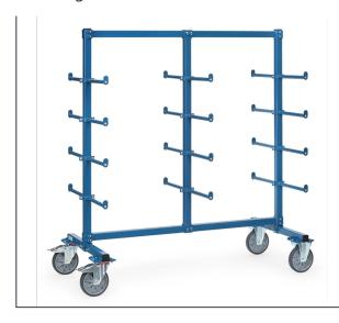
Modular system: Frame made of sturdy square tube. Cross beams, posts and bars connected with solid screwed joints. Carrier spars made of tubular steel Ø 27 mm with screwed joints. With 24 carrier spars on both sides (12 per side) coated with PVC hose and with anti skidding device. Carrying capacity per level 120 kg (60 kg per side). Powder coated blue RAL 5007. 2 swivel and 2 fixed-wheel castors, TPE tyres, hubs with groove ball bearing. Swivel castors with wheel locks, according to EN 1757-3.
